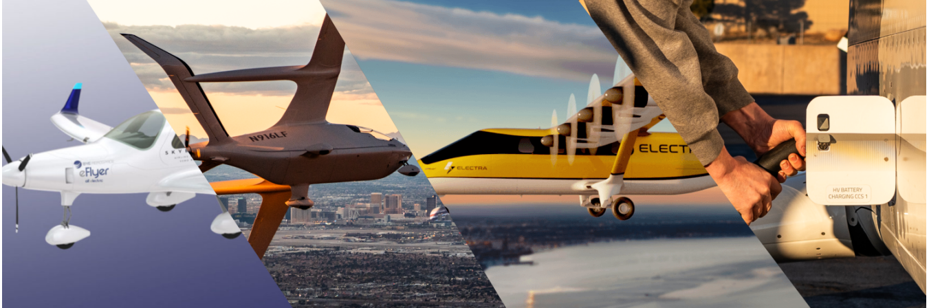
Figure 1: In development and currently available electric aircraft. From left to right, Bye eFlyer2 [4], Beta CTOL [5], Electra EL9 [6], and the CCS charging interface for a BETA aircraft [5].
