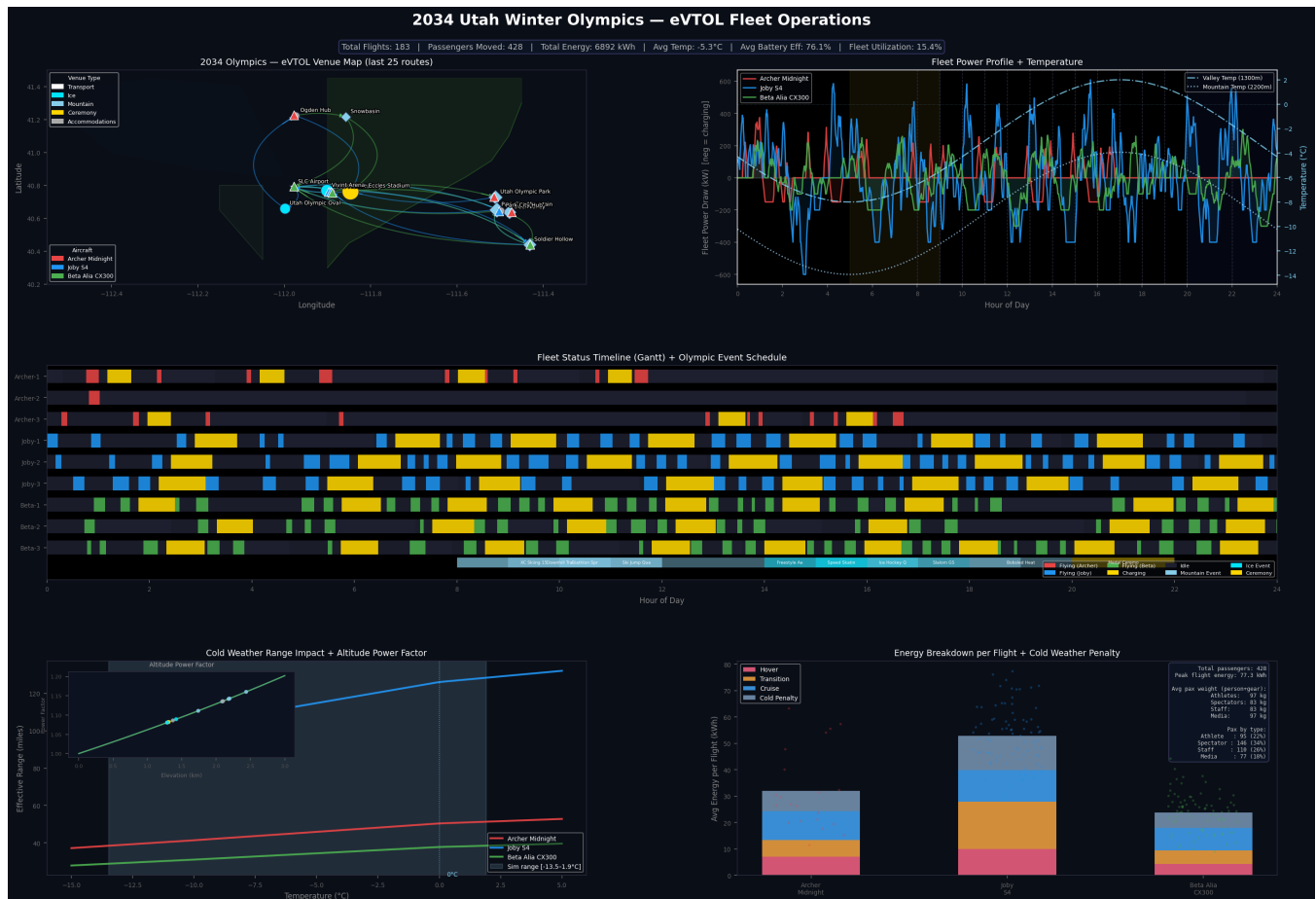
Figure 6: Full 24-hour fleet operations dashboard. Top-left: Venue map with recent flight arcs. Top-right: Fleet power profile (positive = discharge, negative = charging) overlaid with valley and mountain temperature curves. Middle: Per-aircraft Gantt chart (flying / charging / idle) with Olympic event schedule. Bottom-left: Cold-weather range reduction and altitude power factor curves. Bottom-right: Per-phase energy breakdown with cold penalty and passenger statistics.
