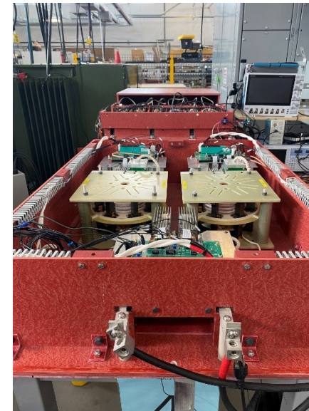
4.16 kV 3-phase AC, 560 kW modular DC fast charger.
