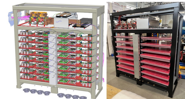
System hardware layout for the 1 MW wireless charging pilot at Utah Inland Port.
